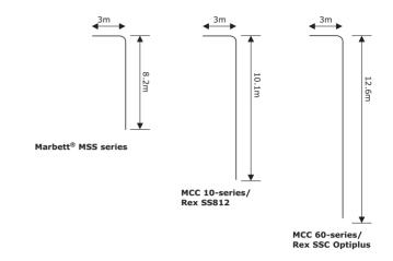
Looking at an L-shaped conveyor with a 90 degree curve, running with 1.5 ltr PET bottles.
